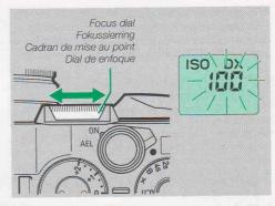
2 Turn the focus dial until either "DX" or the desired film speed appears.
