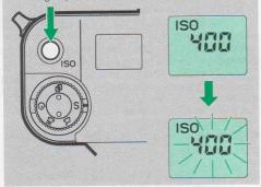
Turn the main switch on. If you press and hold on the ISO button for about 1.2 seconds or more, the display of the film speed in the display panel will start to blink.
