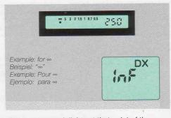
The focusing mark lights at that point of the distance scale indicating the distance at which was focused. Simultaneously, the distance is indicated on the display panel.
