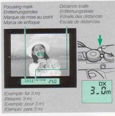
2 Aim the focusing frame at your subject; and depress the shutter release half way. As focusing is performed automatically, the focusing mark will light in the viewfinder.
