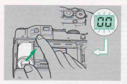
As soon as the entire roll of film is exposed, the camera rewinds the film automatically.
